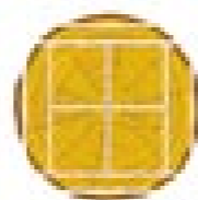
cross section of quarter-sawn timber
